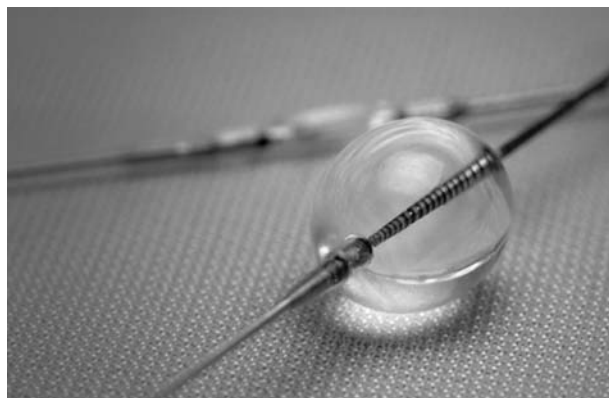
Figure 10.3 PercuSurge GuardWire temporary occlusion and aspiration system.
